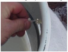
3. Plug the sensor cable into the Remote Ready dial and transmitter cable.
