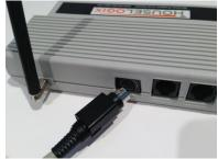
3. Plug in provided power supply to receiver.
